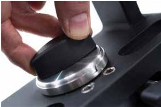
**Jockey Wheel Removal:** Fully remove the jockey wheel caster lock nut <sup>[Fig. 10]</sup>, hold jockey wheel assembly and lift the Jackal chassis away <sup>[Fig.11]</sup>.
